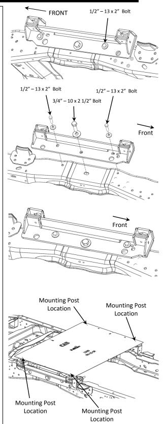
WARNING: Prior to drilling any holes, be sure to check the inside of the frame to guard against drilling into the fuel tank, wiring, brake lines or fuel modules.
