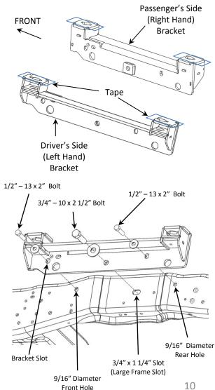
c. Take (1) ½" – 13 x 2" bolt and ½" flat washer and place it thru the 9/16" dia rear hole. Loosely secure the bolt and washer with ½" flange nut.
