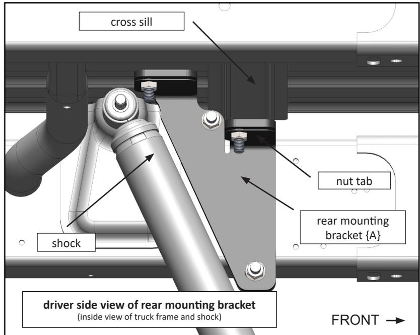
8. Remove the Rear Mounting Brackets and drill out the five (including center base rail hole) rear mounting bracket pilot holes with a 9/16" drill bit.
