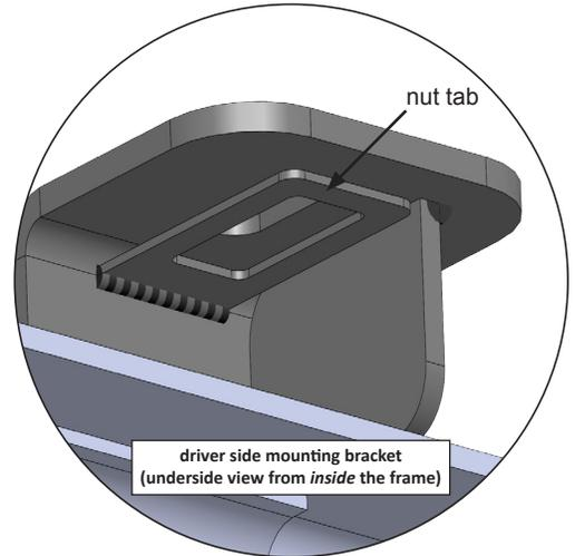
**INSTALLATION TIP:** Prior to threading the Spline Bolt into the leader, thread the 1/2" Flange Nut {L} on and off the bolt to assure that the nut will fit easily once the bolt is in place.
