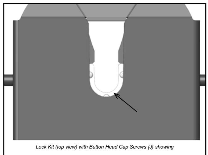
Lock Kit (top view) with Button Head Cap Screws {J} showing
